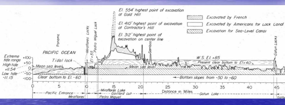
The deepest excavations for the Panama Canal were concentrated near the Continental Divide, as shown in this vertically exaggerated section.
