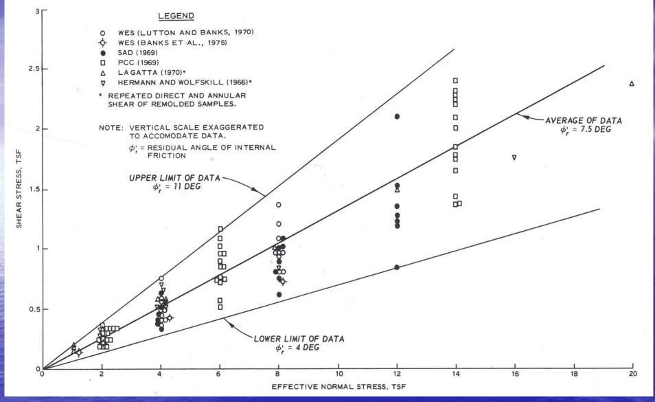
By 1974, the Corps of Engineers decided that the best graphical method to describe strain softened materials was to use a fan plot, showing the upper and lower limits of strength.
