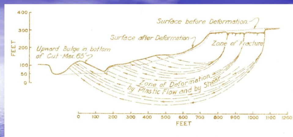
IDEAL CROSS-SECTION WEST SIDE GAILLARD CUT, NEAR CULEBRA, TO SHOW DEVELOPMENT OF DEEP DEFORMATION TYPE OF SLIDE IN CUCARACHA ROCKS.
