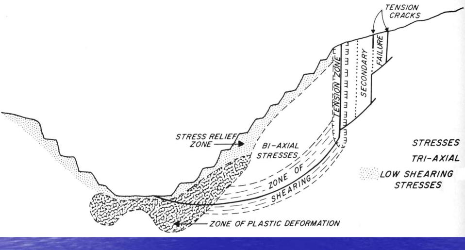
By the mid 1940s Corps of Engineers researchers were beginning to appreciate the significance of stress regimes and strain on soil strength parameters, as sketched here.
