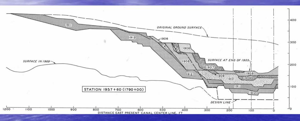
Successive sections through the East Culebra Slide. Note original ground surface and surface in 1969.
