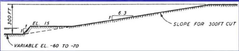
In 1947 the Corps evolved the first design charts for the most problematic units along the canal; these are for the Cucaracha Shale
