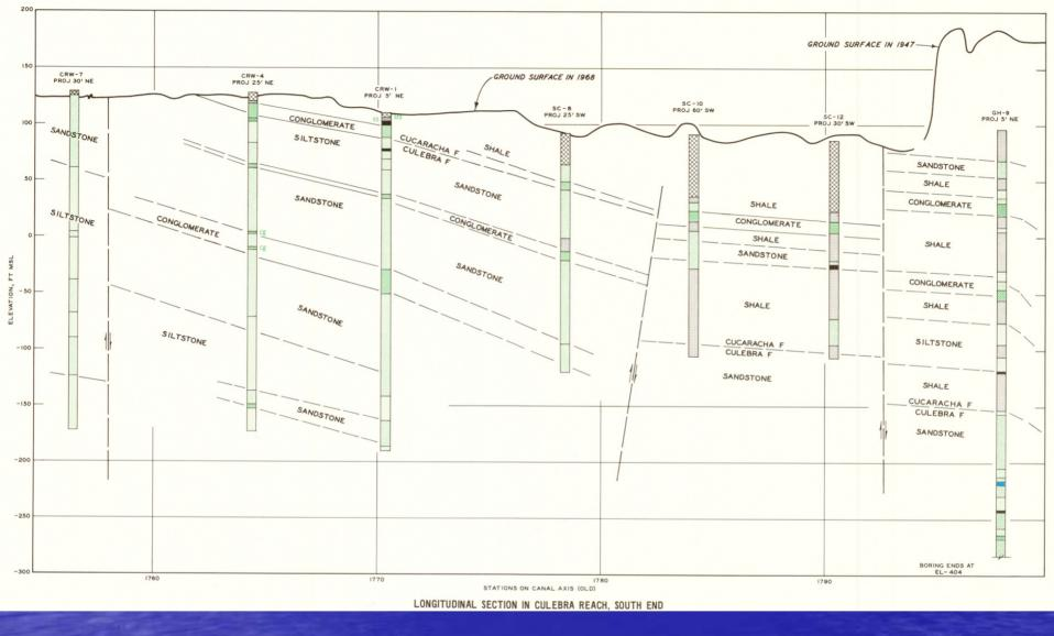
Longitudinal section at south end of Culebra, where slides encroach both sides of the canal.
