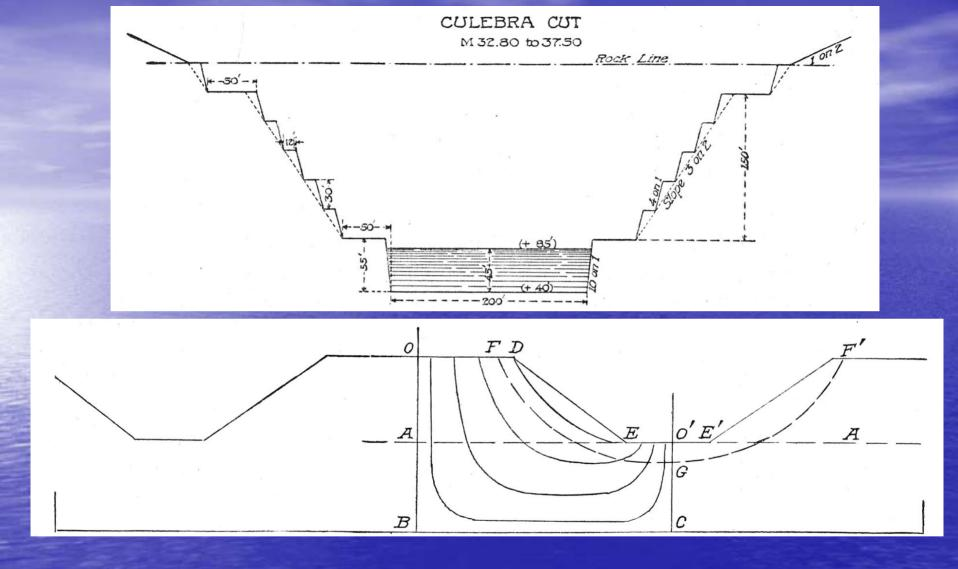
• The 1924 NAS study did a credible job of documenting the history of landslide problems along the canal excavations, but offered little in the way of meaningful analyses or solutions. Note flow net.
