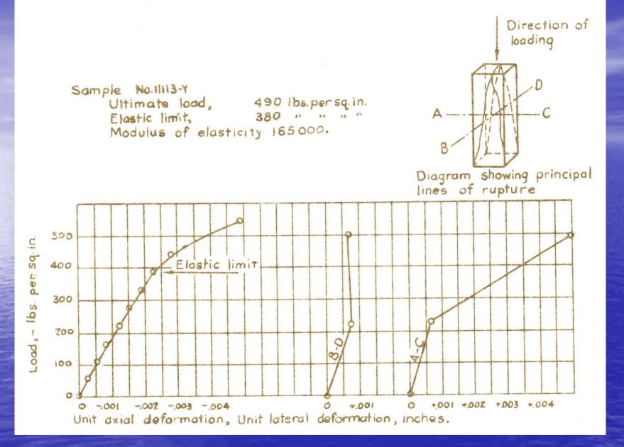
Early compressive strength tests on the Culebra formation
