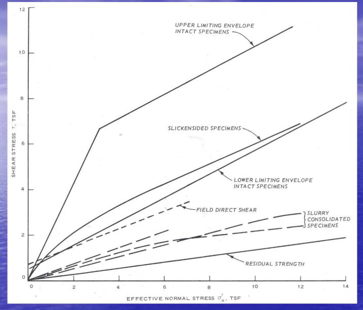
Shear vs effective normal stress plots. Note impact of disturbance, or plastic strain, on mobilized shear strength.
